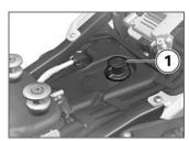
Remove cap from oil fill location 1 by turning counterclockwise.
